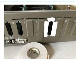
Step 2: Fold the NEWPRINT end of the ribbon cable at a 45° angle as shown.
