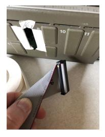
Step 3. Feed the ribbon cable from inside the Apple II through the rear port.
